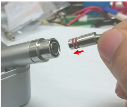
Step1. Insert tip onto handpiece.
