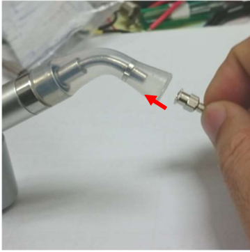
Step4. Insert root canal tip onto air tip.
